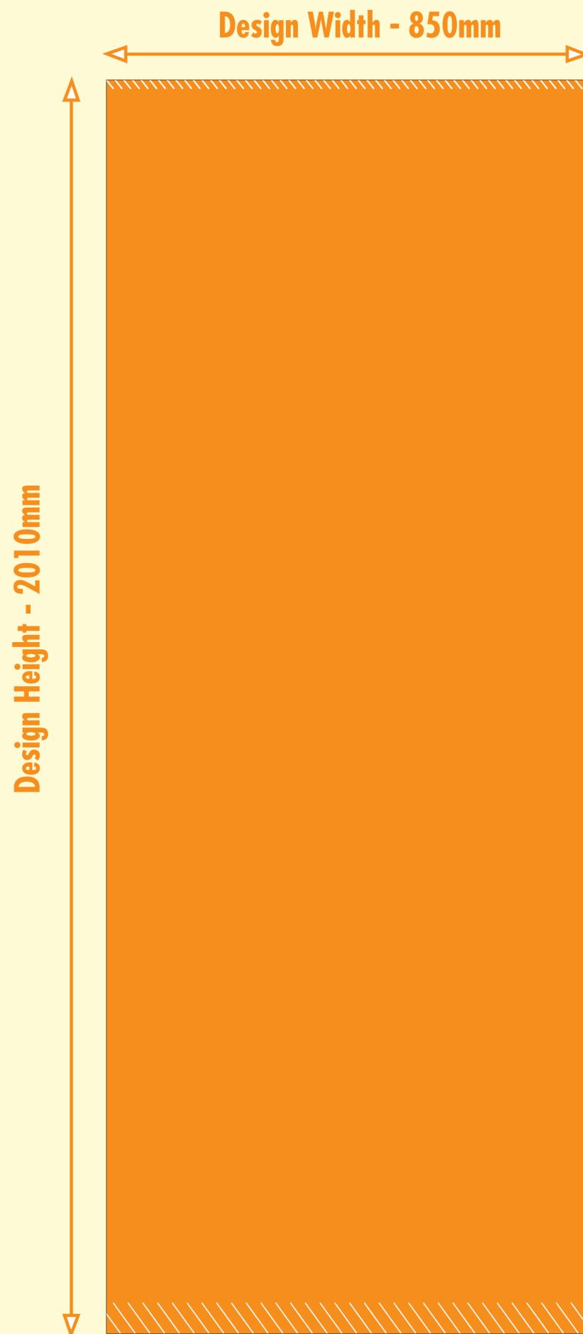
The top 15mm are used to house the top bar...
